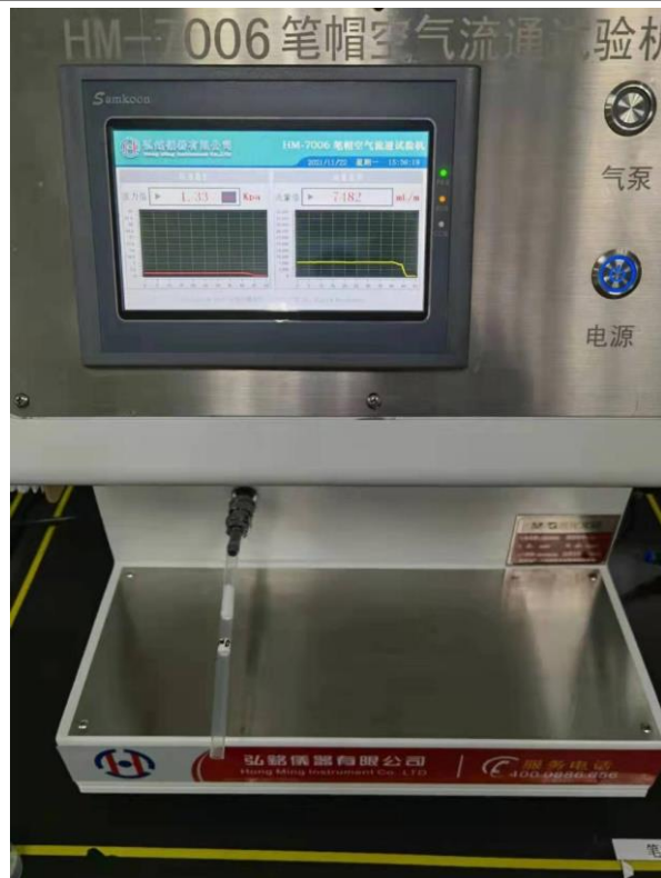
Air Circulation Test Machine for Pen Caps
